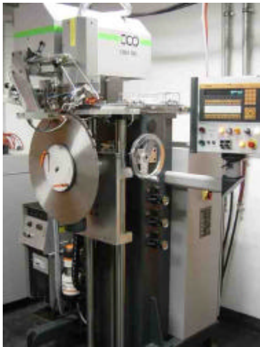
Fully automatic brazing machine for circular saw blades
