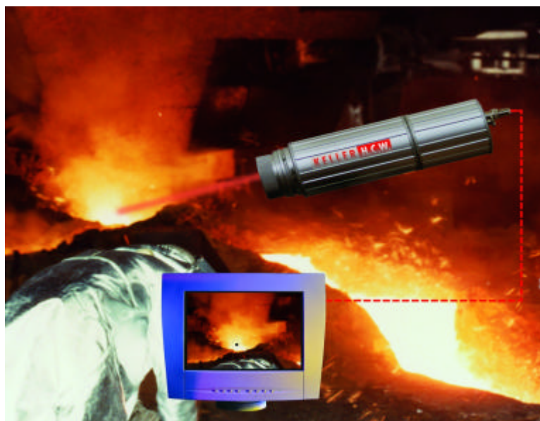
Photo 5: Temperature Measurement with Video Surveillance at the transfer channel of a blast furnace
