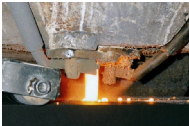
Photo 1: Pour stream at an automated casting line
