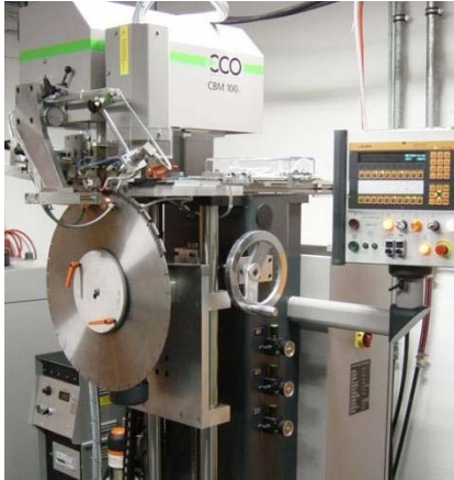
Fully automatic brazing machine for circular saw blades
