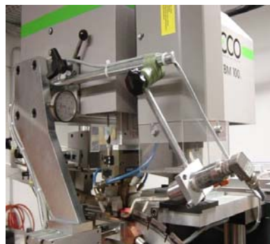
The pyrometer detects the temperature precisely at the target spot
